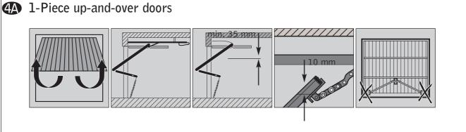
Install door bracket at centre position of door and rail bracket on centre position above door. Make sure there is at least 10 mm clearance between highest travel point of door and rail.
