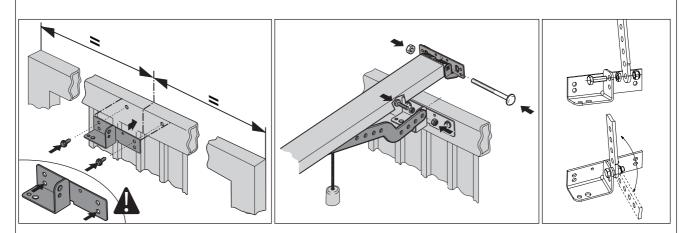
▲ For doors fitted with 3 point latching: Before fitting the door bracket to the door, the top latch assembly must be removed. For GRP doors only —also remove the retaining screws alongside the door bracket fixing holes. When fitting the door bracket, use the lower holes for GRP doors only and the upper holes for all other doors.
